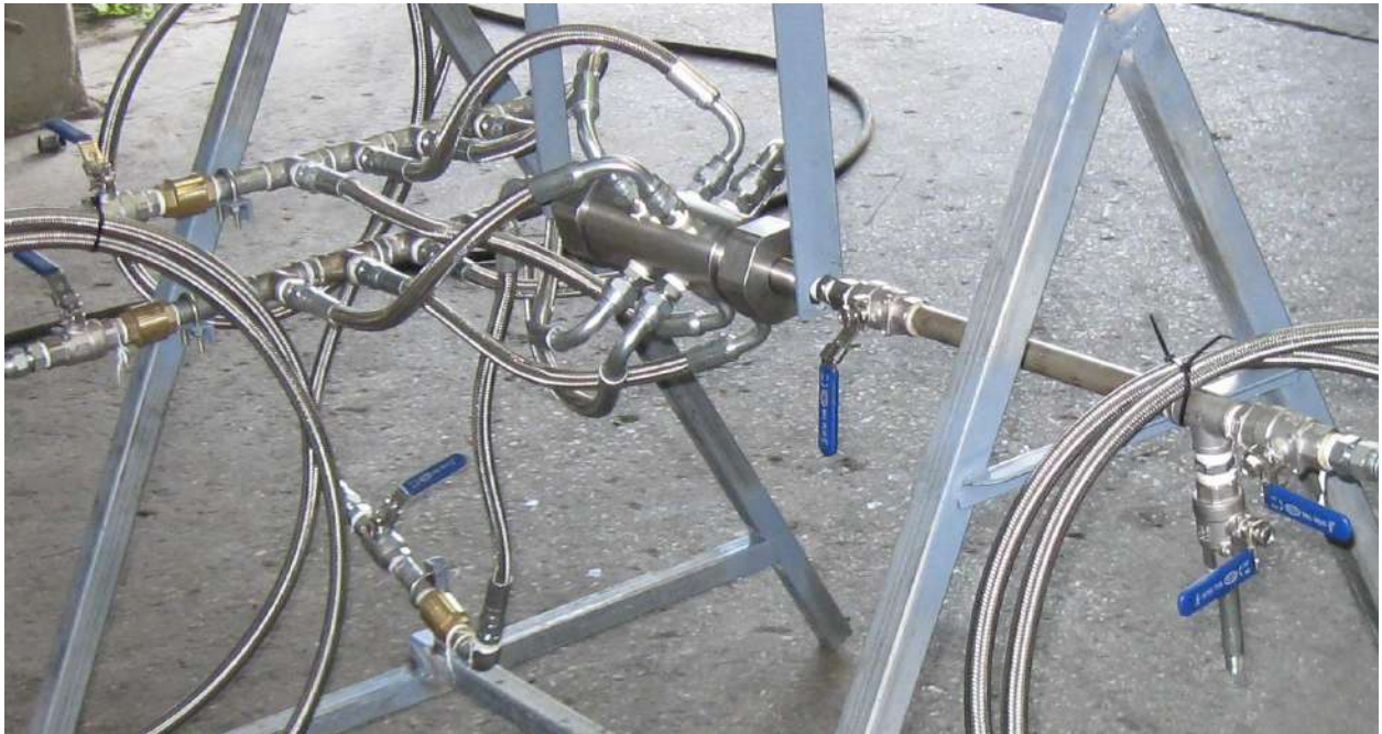
Industrial system for dynamic mixing and homogenization with maximal flow = 1000 liter per hour, under maximal pressure 30 bar
